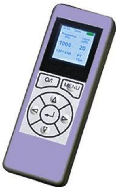
The Kamplex KMS-1 is a high specification screening Free Field and Puretone audiometer (using optional TDH39 headphones or E5A insert earphones) in a handheld format the size of a mobile phone.
