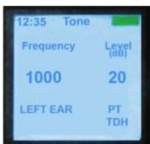
This example screen displays current test parameters set up using the relevant menus. The top line is the status line which shows current time and battery level. It also indicates when the 'present' button is pressed.
