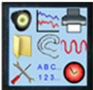
The main menu screen displays icons for the different functions on the KMS-1. This menu screen is always accessed with the menu key on the keypad. Each function is easily selected using the four arrow keys and enter key. Sub-menus can then be selected to set up the necessary parameters.
