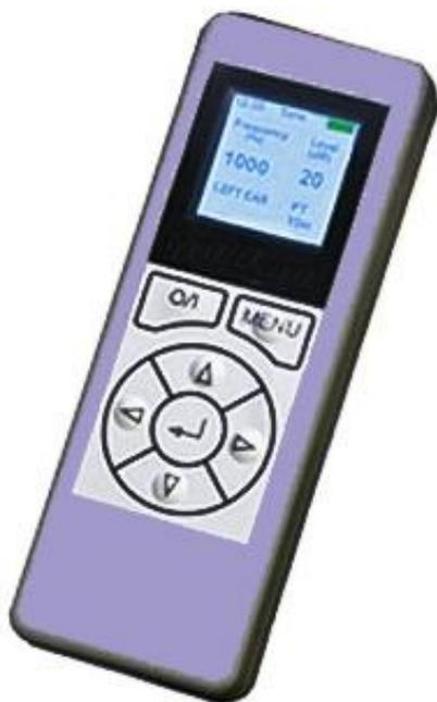
The Kamplex KMS-1 is a high specification screening Free Field and Puretone audiometer (using optional TDH39), in a handheld format the size of a mobile phone.
