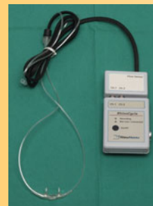
Fig. 2: Data logger with tubes and pressure transducers
